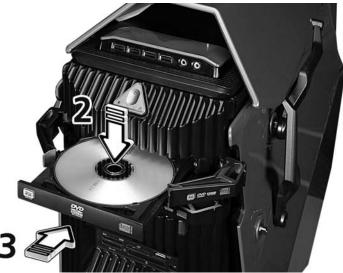
3. Push the tray and it will close automatically or press the eject/load button.
